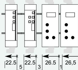
To insert the  $\mu$ console : mount the instruments vertically (on horizontal DIN rail) and provide a 5mm space-ment.
